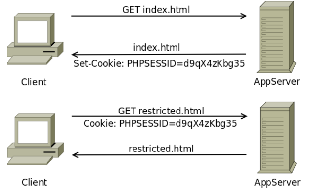
Fig. 1. Top: creation of a new session in the first response from the server to the client. Bottom: attaching of the SID to subsequent requests from the client to the server.
