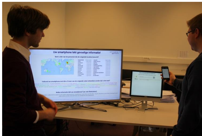
Fig. 1. The setup, as it was deployed at our research institute. The main screen, displaying aggregate information about all smartphones in a range of 50 meters is shown on the left. To the right of this screen is another (smaller) screen, on which a smartphone user can choose to display the information our system gathered from his/her smartphone.
