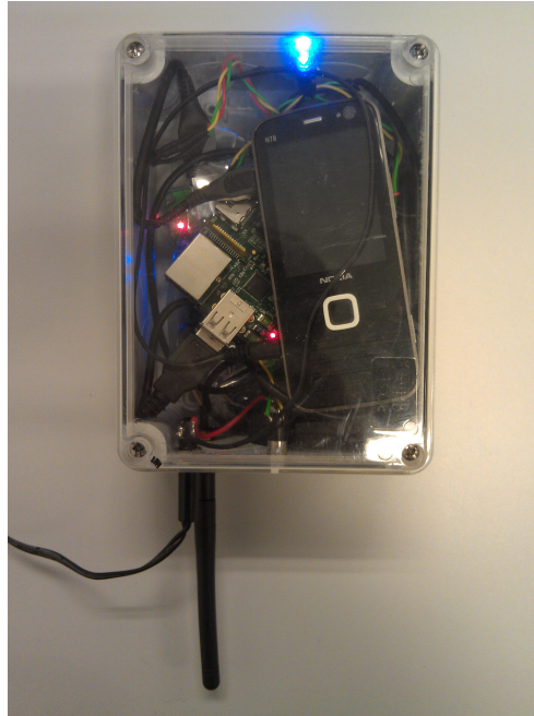
Figure 2.3: The Wi-Fi detector, consisting of: (a) a Raspberry Pi, (b) a Wi-Fi dongle, (c) an external long-range antenna, (d) a USB hub, (e) a Nokia N78 phone, and (f) a heartbeat LED.
