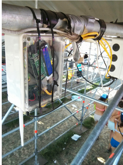
Figure 2.5: The second version of the Wi-Fi detector, installed at Pukkelpop 2013, also containing an LCD display.
